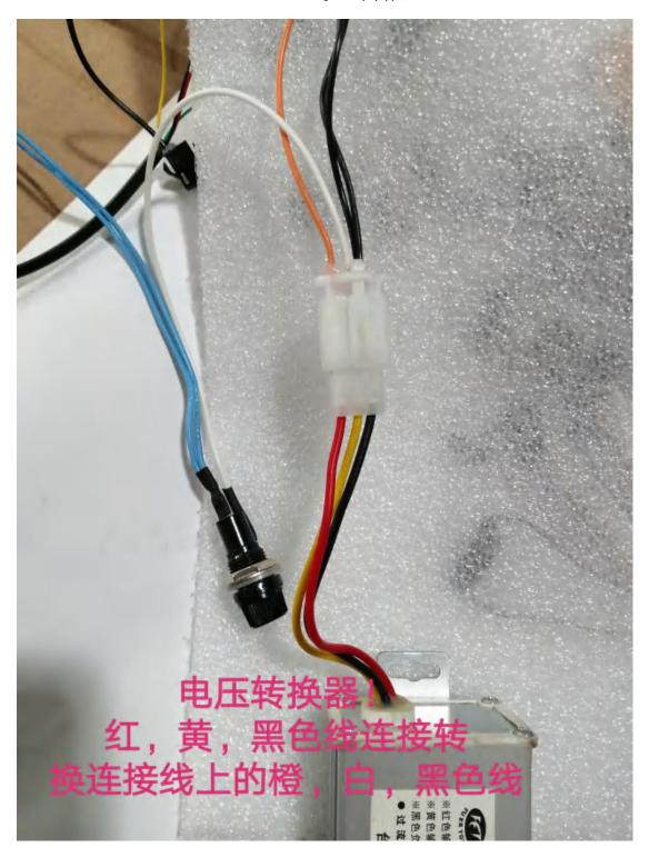
Connect the black, red and yellow lines with the black, orange and white lines from the conversion cable. It is the voltage converter.
