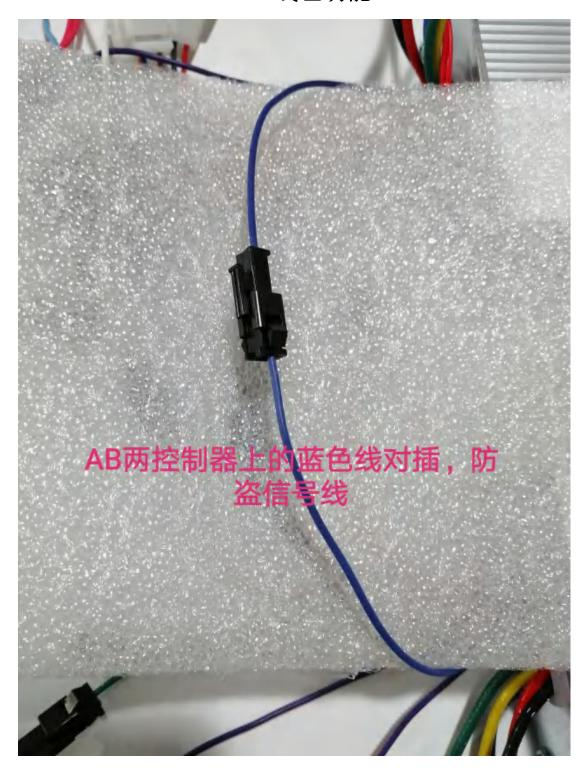
Connect the blue lines of the A controller and B controller. It is the anti-theft signal line.
