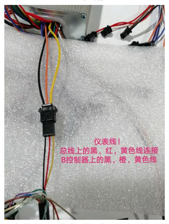
Connect the black, red and yellow lines from the wire with the black, orange and yellow lines from the B controller. It is the display line.
