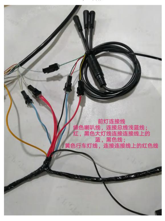
Headlight connection line Connect the green speaker line with the light blue from wire. Connect the black light line with the blue and black lines from connection line.
