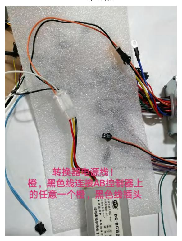
Converter power cord Connect the orange and black lines with orange and black lines from A controller or B controller.
