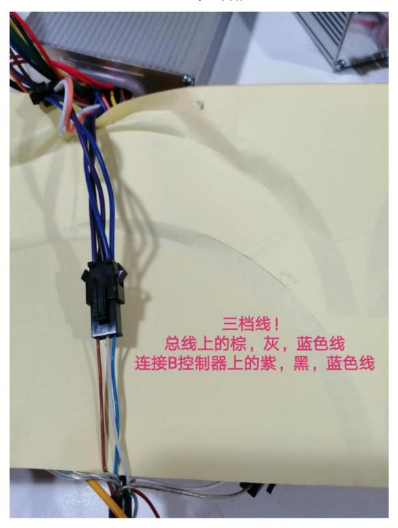
Connect the brown, grey and blue lines from the wire with the purple, black and blue lines from the B controller. It is the brake signal line.
