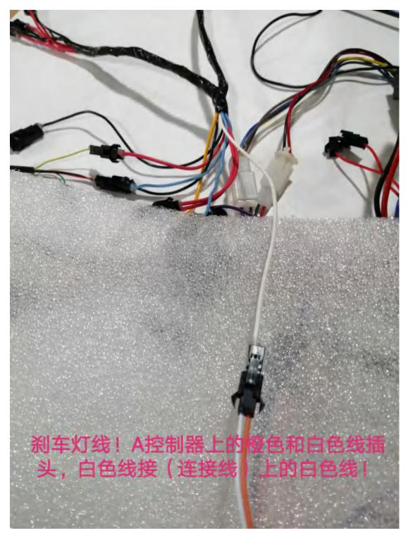
Connect the orange and white lines of the A controller and white line of the connection line. It is the brake light line.
