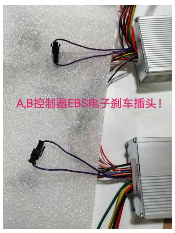
Electronic brake plug (EBS) from A and B controller. Connect it as the picture.
