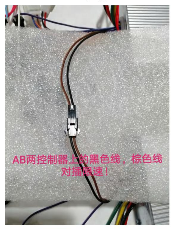
Connect the black and brown lines of the A controller and B controller. The functoin is speed limitation.
