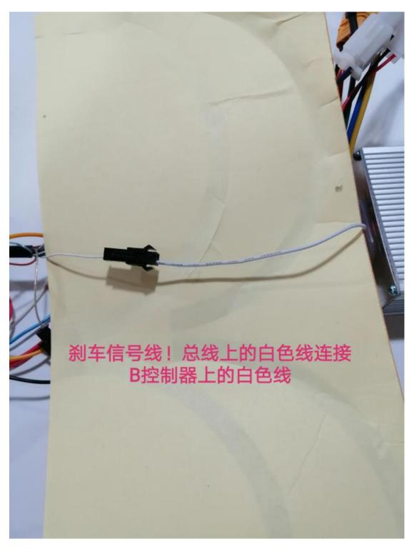
Connect the white line from the wire and the white line from the B controller. It is the brake signal line.
