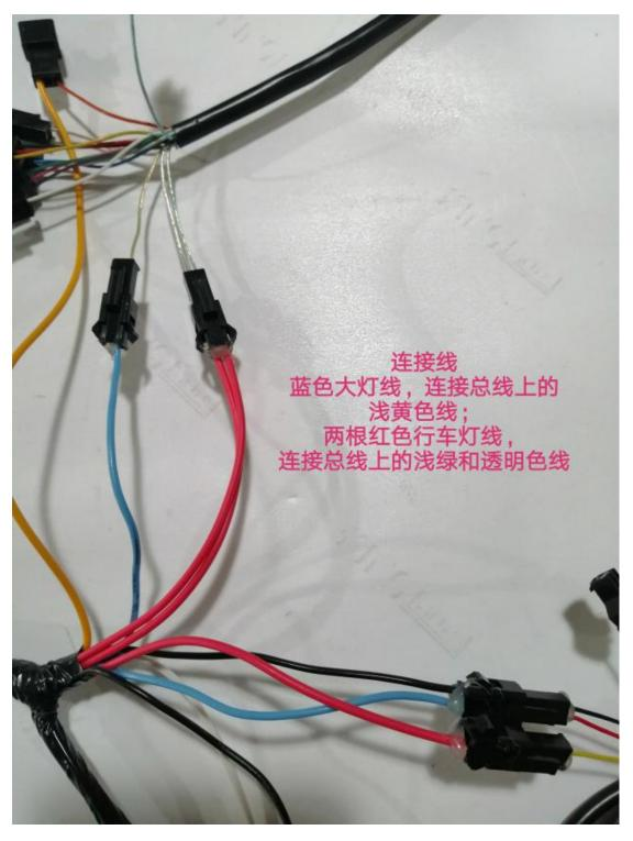
Connection line Connect the blue light wire with the light yellow line from the wire. Connect two red bike lights with the light green and sliver line.
