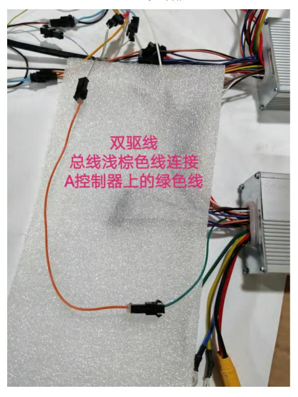
Dual drive line Connect the brown line from wire with the green line from the A controller.
