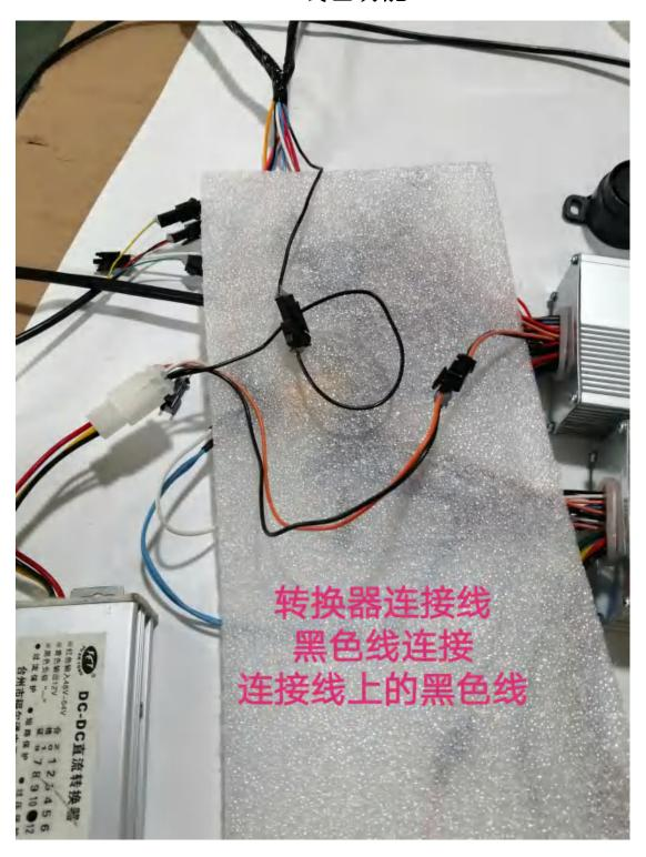
Converter cable Connect the black line with black line from connection line.
