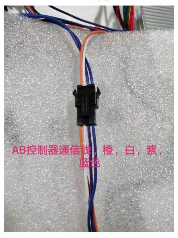
Connect the orange, white, purple and blue lines of the A controller and B controller. It is the communication line.
