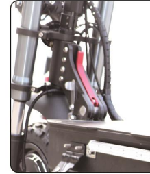
Quick folding mechanism self locking/release grip
